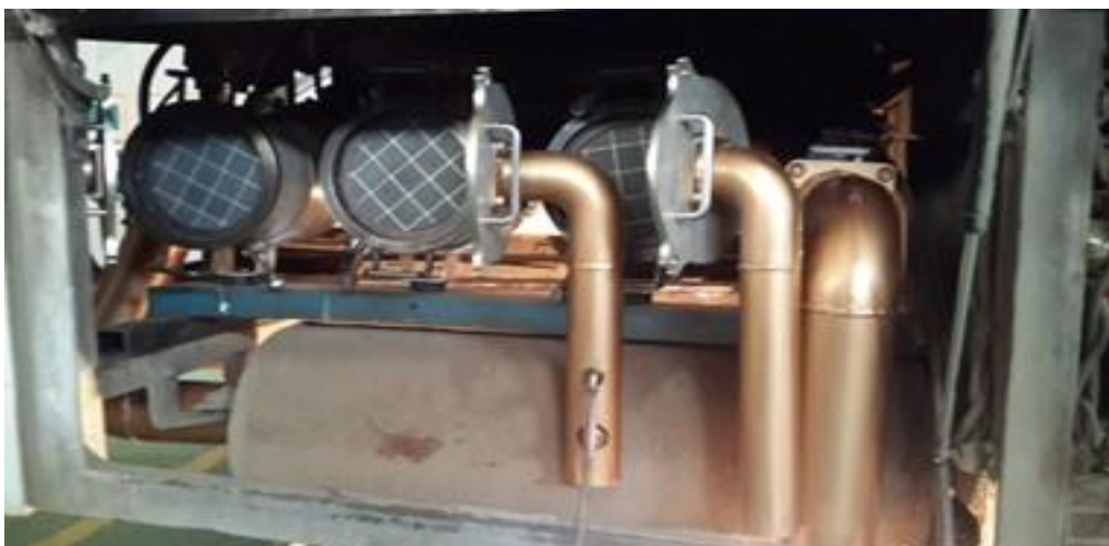
Figure 3. DPF system installed on DAEWOO BS106 bus
