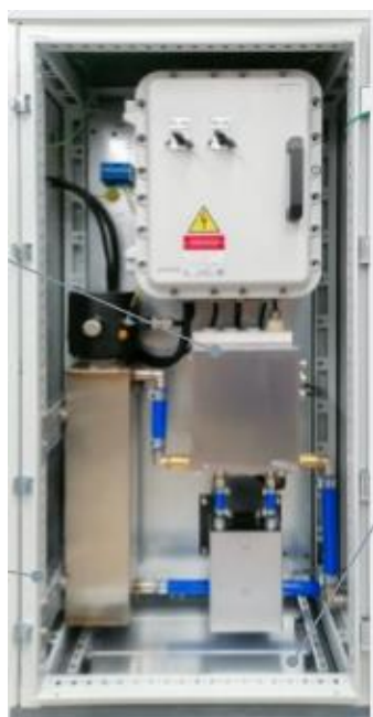
Fig. 2. A system for the automatic measurement of drilling fluid parameters
